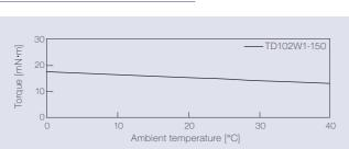
The torque achieved during rotation at 20 min<sup>-1</sup> in the designated ambient temperature is shown.
