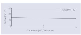
Measurement of torque at a rotation speed of 20 min<sup>-1</sup>
